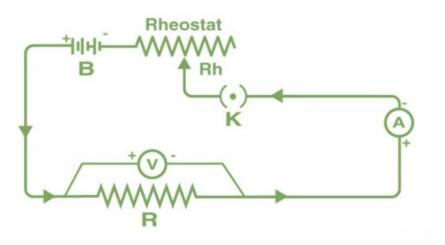
Ohm's Law isn't just a theory; we can put it to the test! Here's how to conduct an experiment to verify this law:
